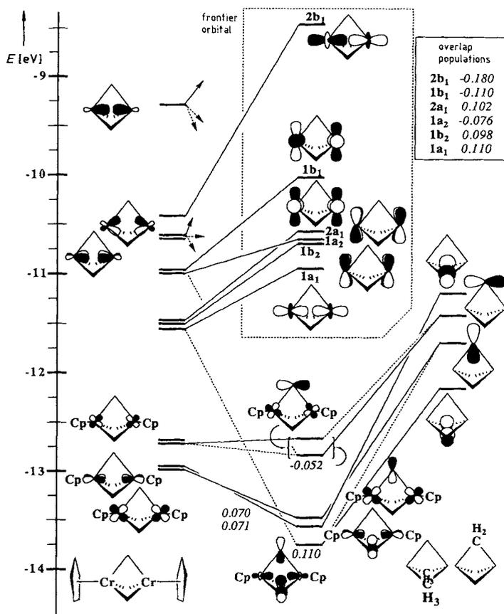
Fig. 2. Partial interaction diagram for  $\{[\text{CpCr}(\mu\text{-CH}_3)]_2(\mu\text{-CH}_2)\}$  (**2a**). Numbers in italics are overlap populations; symmetry labels were assigned assuming  $C_{2v}$  symmetry. The overlap populations for the frontier d orbitals (inner box) were calculated for doubly occupied levels. Cp denotes substantial charge density on the cyclopentadienyl ligand.
