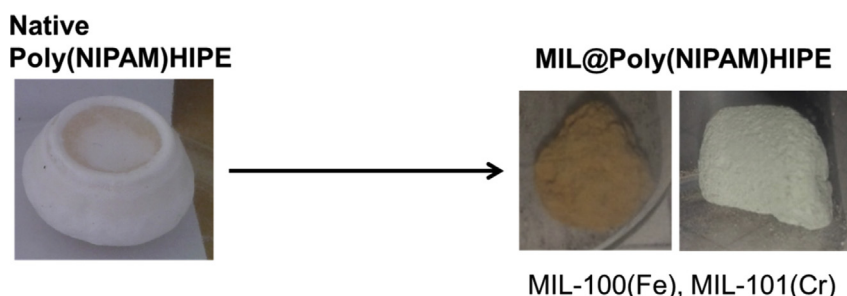
Scheme 3. Synthetic route to synthesize MIL@poly(NIPAM)HIPE (MIL-100(Fe,Cr), MIL-101(Cr)). Only MIL-100(Fe)@NIPAM and MIL-101(Cr)@NIPAM composites are shown.
