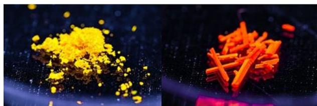
**Figure 4.** Solid state fluorescence of 6-aryl-8*H*-indolo[3,2-*a*]phenazines **18a** (left) and **18e** (right);  $\lambda_{\text{ex}} = 365\text{ nm}$ .
