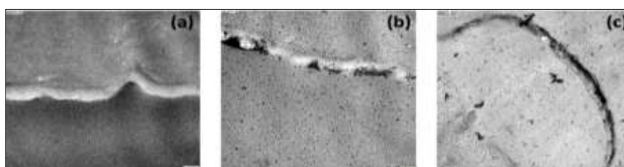
Fig 11: TEM images of non-impregnated (a), simple soaking impregnated (b) and in situ impregnated (c) cotton material with Cymbopogon citratus -mediated silver nanoparticles.
